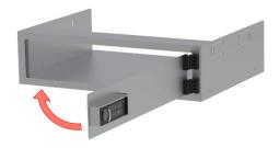
2. Press any numeric key once and turn the rotary opening handle counterclockwise by 90° into the "closed" position (the lock closes automatically).
